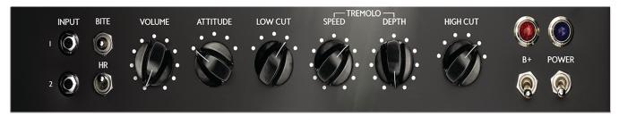
INPUT I is tailored to a single coil pickup and INPUT 2 to a Humbucker, but you can run whatever you like into either.
